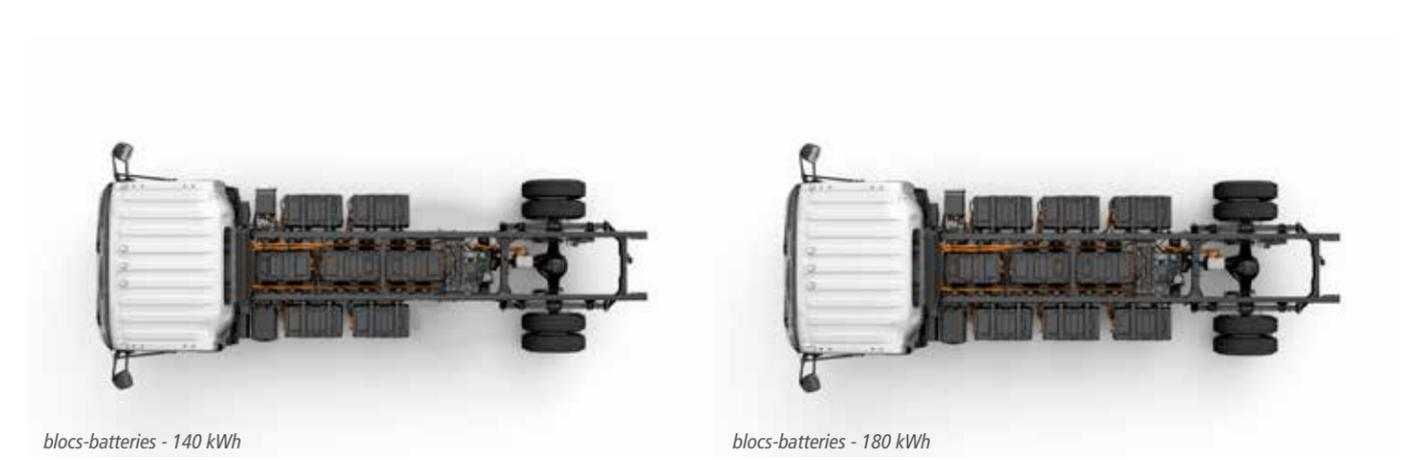
blocs-batteries - 140 kWh
